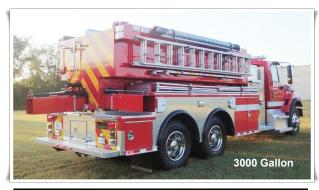
Tanker Bodies are built with Heavy Duty All Aluminum Extruded Construction.
